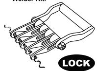
Remove dent by gradually working Magna Claw over length of crease. Pull until all fingers are even.
