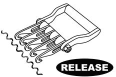
Disengage Magna Claw from wire and complete repair.
